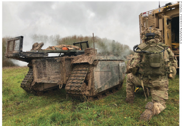
THE MODULAR BASE can be adapted for various missions, including casualty retrieval.
